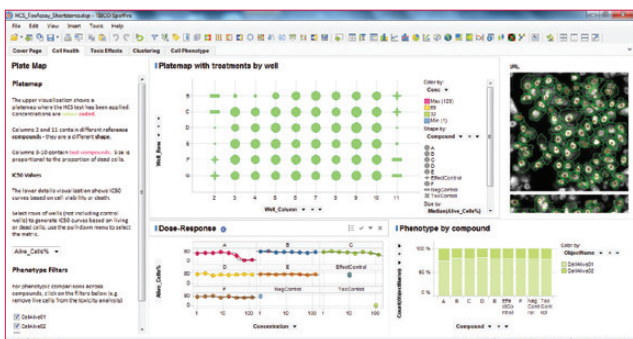
TIBCO Spotfire® Pro client showing a cell toxicity study: the tab pictured is summarizing cell health. The plate map controls what other data is displayed, including dynamically calculated dose response curves and the stored cellular images.
